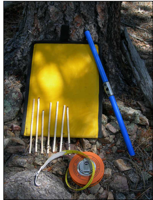
Figure 5. Field measurements of tree diameter and site index were made with a diameter tape (orange) and increment borer (blue).
